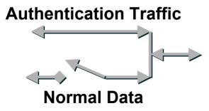
AP "Encapsulates" 802.1x Traffic into RADIUS Traffic, and Visa Versa
